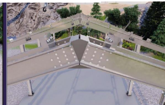
CENTRAL CONNECTION DETAIL
