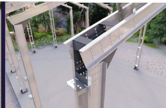
CORNER CONNECTION DETAIL
