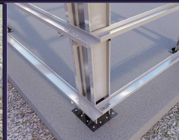
WALL- PURLIN CONNECTION DETAIL
